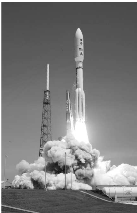
▲ FIGURE 1.2. This is NASA's Juno planetary probe launching atop an Atlas V rocket. About one minute after takeoff, a rocket like this will have traveled through the 100 kilometers (about 62 miles) of Earth's atmosphere and be in empty space.
